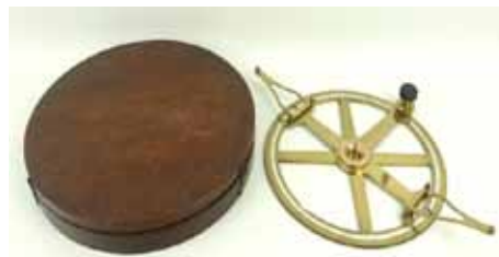
1017 A late 19th century brass circular protractor by William & John Cary, London, with two brass folding radius arms inscribed 'Cary, London' and vernier scale, 7 inch radius, external teeth and worm gear for adjustment, 19.5cm across, in a fitted circular mahogany case with hook and eye latches, 3.5 by 24cm. £150 - £250
