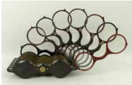
1085 A late 19th century optician's folding lens testing set in a horn frame, comprising eight numbered lenses. £30 - £50
